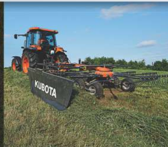
RA Series Rotary Rakes 13'9" working width with rugged, high-lift tine arms
